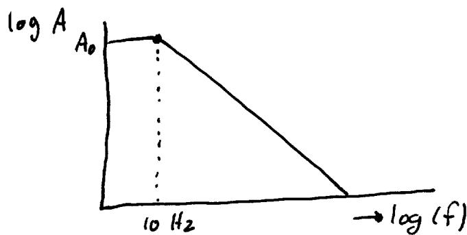
with a cut-off frequency at 10 Hz. The transfer function of this is
