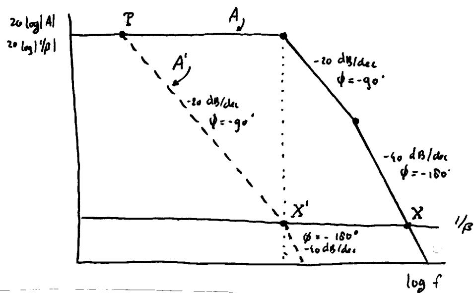
In the above figure : by introducing a new pole  $P$  at low frequencies the gain is reduced to below  $1/\beta$  before the phase changes of the other poles take effect. To be sure this works for any  $\beta$ , a  $\beta$  of 1 has to be used in the calculation for the design of  $P$ .
