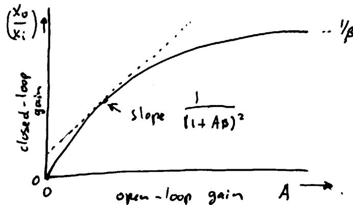
The relative change in gain is thus related to the relative <sup>change in</sup> gain of the open circuit :
