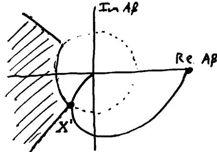
It is not difficult to show that a  $\beta = 10^{-3}$  is needed to stabilize the circuit. For example with  $R_1 = 100 \Omega$  and  $R_2 = 100 k\Omega$ .
