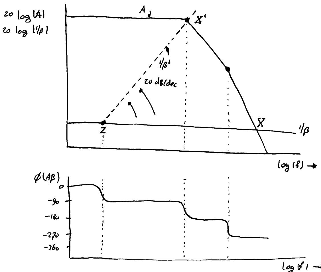
By the zero  $Z$ , the  $1/\beta$  is pushed up to make it cross with  $A$  earlier, before the first pole of  $A$ .
