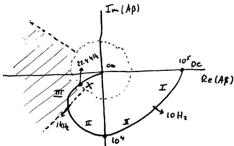
Conclusion : The circuit runs the risk of oscillating in the frequency range  $1 \text{ kHz} - 22.4 \text{ kHz}$
