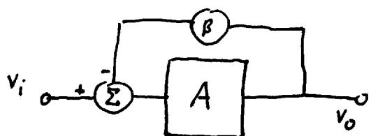
$$\left. \begin{array}{l} A = 10^4 \\ \beta = \end{array} \right\} \frac{V_o}{V_i} = \frac{A}{1 + A\beta} =$$
