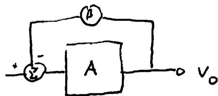
Also here we can see that if  $A\beta = -1$  then the output will be infinite for any tiny voltage at input. Normally, noise is present at any point of the circuit ( $\sim \mu V.. mV$ ) and this will initiate the oscillations.
