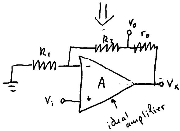
$$\frac{V_x}{V_i} = \frac{A}{1 + A\beta'} , \quad \beta' = \frac{R_1}{R_1 + R_2 + r_o}$$
