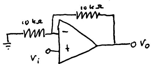
A has two poles, 10 Hz and 1 kHz. The DC gain is  $+10^5$ . Will this circuit oscillate? If so, at
