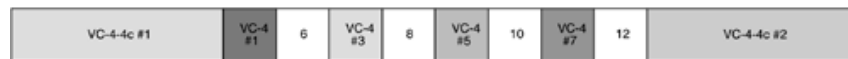
(c) STM-16 (OC-48) signal with two VC-4-4cs (STS-12cs) and four VC-4s (STS-3cs)
