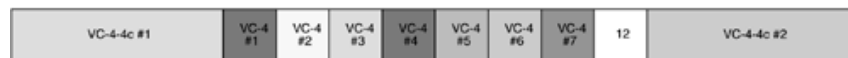
(b) STM-16 (OC-48) signal with two VC-4-4cs (STS-12cs) and seven VC-4s (STS-3cs)
