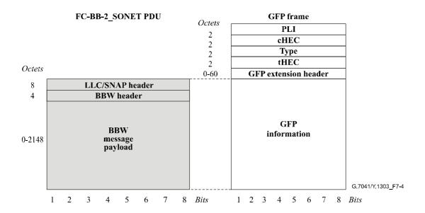
Figure 7-4/G.7041/Y.1303 – Fibre Channel Broadband-2 SONET (FC-BBW\_SONET) and GFP frame relationships
