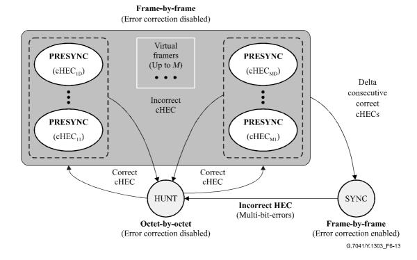
Figure 6-13/G.7041/Y.1303 – GFP frame delineation state diagram
