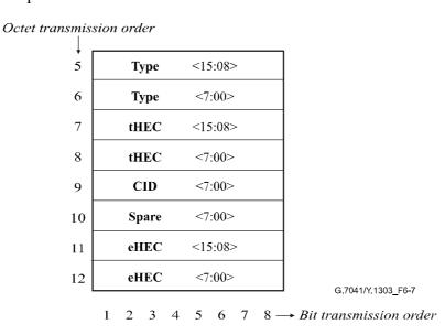
Figure 6-7/G.7041/Y.1303 – Payload header for a linear (point-to-point) frame including the extension header
