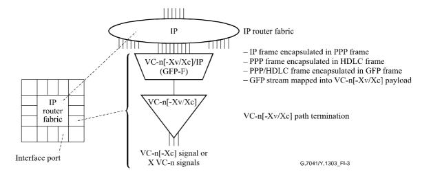
Figure I.3/G.7041/Y.1303 – VC-n/VC-n-Xv/VC-n-Xc port on IP router, or IP router function embedded in hybrid SDH/IP equipment
