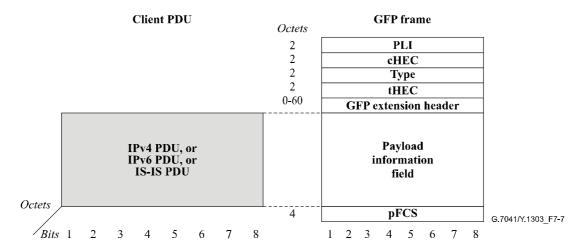
Figure 7-7/G.7041/Y.1303 – IPv4/IPv6/IS-IS PDUs and GFP frame relationships
