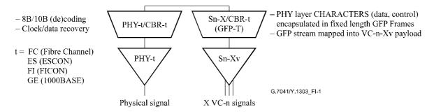
Figure I.1/G.7041/Y.1303 – FC/ES/FI/GE tributary interface port using full-rate GFP-T mapping in SDH network element
