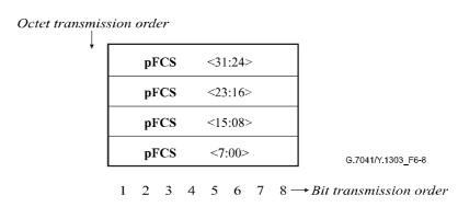
Figure 6-8/G.7041/Y.1303 – GFP payload frame check sequence format
