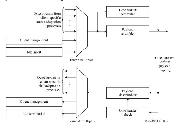
Figure 6-12/G.7041/Y.1303 – GFP Common (Protocol Independent) Procedures
