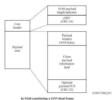
Figure 6-1/G.7041/Y.1303 – Frame format for GFP client frames
