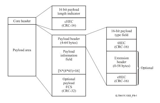
Figure 8-1/G.7041/Y.1303 - Transparent GFP frame format
