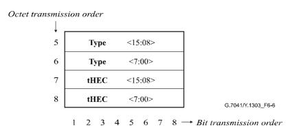
Figure 6-6/G.7041/Y.1303 – Payload header for a GFP frame with a null extension header
