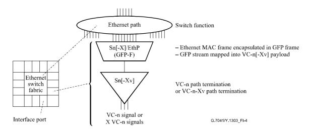
Figure I.4/G.7041/Y.1303 – VC-n-Xv port on Ethernet switch, or Ethernet switch function embedded in hybrid SDH/Ethernet equipment
