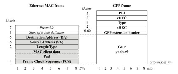
Figure 7-1/G.7041/Y.1303 – Ethernet and GFP frame relationships
