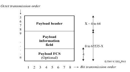
Figure 6-3/G.7041/Y.1303 - GFP payload area format
