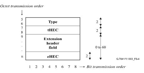
Figure 6-4/G.7041/Y.1303 – GFP payload header format
