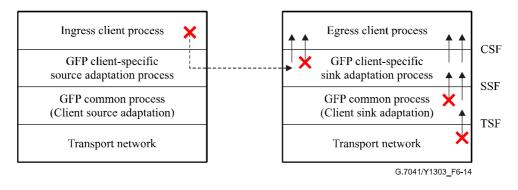
Figure 6-14/G.7041/Y.1303 – Defect signal propagation in GFP
