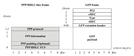
Figure 7-3/G.7041/Y.1303 – PPP/HDLC and GFP frame relationships (with PPP's ACFC configuration option)
