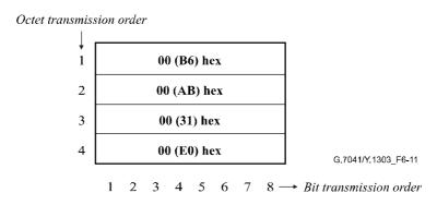
Figure 6-11/G.7041/Y.1303 – GFP idle frame (Barker-like scrambled frame)
