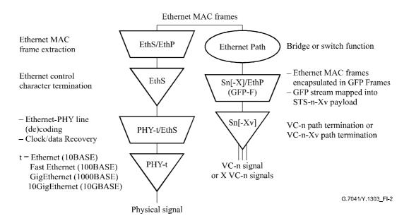
Figure I.2/G.7041/Y.1303 – Ethernet tributary interface port using GFP-F mapping in SDH network element
