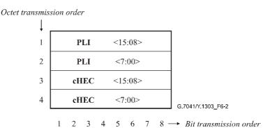
Figure 6-2/G.7041/Y.1303 – GFP core header format
