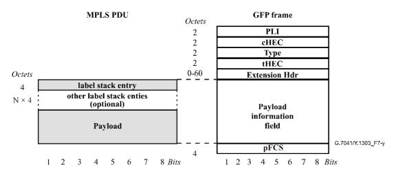
Figure 7-6/G.7041/Y.1303 – MPLS PDU and GFP frame relationships
