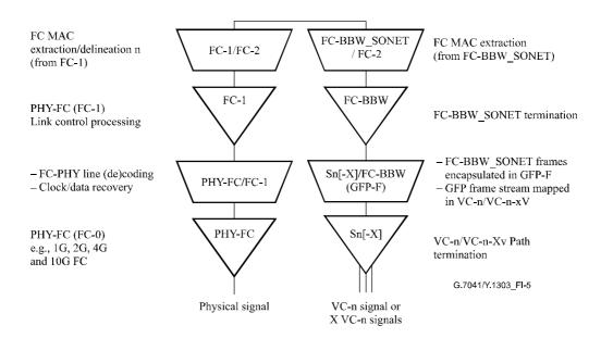
Figure I.5/G.7041/Y.1303 – Fibre channel tributary interface port using FC-BBW\_SONET and GFP-F mapping in an SDH network element
