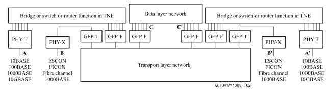
Figure 2/G.7041/Y.1303 – GFP functional model (single client)
