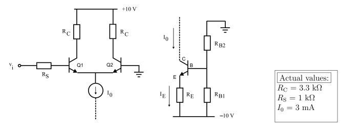
$I_0 = 3 \text{ mA}, I_E = 1.5 \text{ mA}. r_e = 26 \text{ mV} / 1.5 \text{ mA} = 17.33 \Omega. r_{\pi} = 201 \text{ x} 17.3 \Omega = 3.48 \text{ k}\Omega. V_{o2} = V_{o1} = 10 \text{ V} - 1.5 \text{ mA} \text{ x} 3.3 \text{ k}\Omega = 5.05 \text{ V}. r_{in} = 2 \text{ x} r_{\pi} = 7.0 \text{ k}\Omega.$
