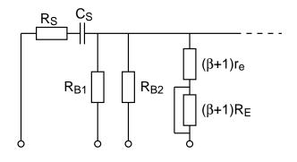
$$\begin{aligned} R &= R_{\rm S} + R_{\rm B1} \| R_{\rm B2} \| (\beta + 1) r_{\rm e} \\ &= 1 \mathrm{k} \Omega + 10 \mathrm{k} \Omega \| 20 \mathrm{k} \Omega \| 6.549 \mathrm{k} \Omega \\ &= 4.304 \mathrm{k} \Omega \\ C_{\rm S} &= 10 \ \mu \mathrm{F} \\ \tau_S &= RC = 43.04 \mathrm{ms} \\ f_{LS} &= \frac{1}{2\pi\tau_S} = 3.7 \mathrm{\,Hz} \end{aligned}$$
