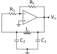
The above circuit is a Colpitts Oscillator. It consists of an ideal opamp with negative feedback composed of R1 and Rf, and a branch with positive feedback, composed of two capacitors and an inductor.
