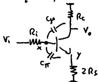
The gain between  $V_x$  and  $V_o$  is  $-0.234$  (for Miller effect). The gain between  $V_x$  and  $V_y \approx 1$ . We get at the entrance the following equivalent circuit:
