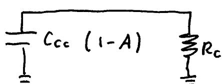
Output resistance  $r_o$  of transistor can be ignored.
