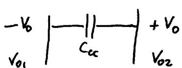
shorted (at high frequencies a capacitor is a short circuit), the outputs are both 0. (the only value that follows the symmetry rules  $V_{o1} = V_{o2}$  and  $V_{o1} = -V_{o2}$ )
