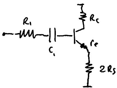
$C_i$  is part of a high-pass filter (HPF).
