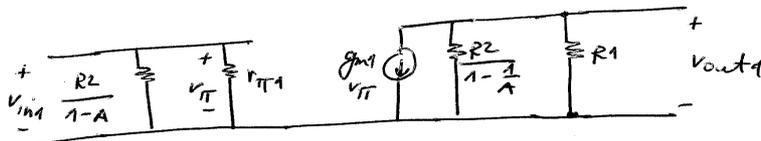
$$\text{com } A = -g_{m1} R_1 = -0.04 \times 9.7 \times 10^3 = -388$$
