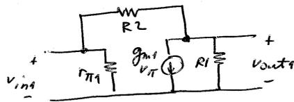
$$\text{com } \frac{1}{r_{\pi}} = \frac{I_B}{V_T} = \frac{1}{\beta} \frac{I_C}{V_T}$$
