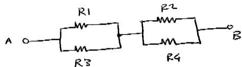
$$R_T = (R_1 \parallel R_3) + (R_2 \parallel R_4)$$
