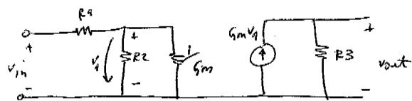
$$\text{Logo } V_{\text{out}} = R_3 G_m V_1$$
