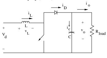
Nominal Values:  $V_{d} = 9 V$  $L = 10 \mu H$  $rL = 10 m\Omega$  $C = 50 \mu F$  $R_{load} = 5 \Omega$  $f_{s} = 100 \text{ kHz}$ switch duty ratio D = 0.625
