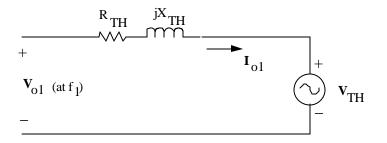
Therefore,  $V_{TH}$  (rms) = 124.1 <u>/-5.39</u>° V and  $v_{TH}$  = 175.5 sin (2 $\pi$ x40xt - 5.39°).
