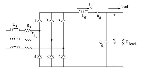
Nominal Values:  $V_{LL} (rms) = 208 \text{ V at } 60 \text{ Hz}$  $L_s = 0.1 \text{ mH}$  $R_s = 1 \text{ m}\Omega$  $L_d = 0.5 \text{ mH}$  $R_d = 5 \text{ m}\Omega$  $C_d = 500 \text{ }\mu\text{F}$  $R_{load} = 16.5 \text{ }\Omega$
