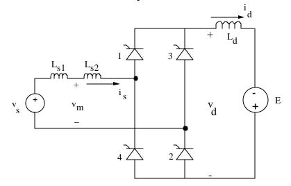
Nominal Values:  $V_{S}(rms) = 120 \text{ V at } 60 \text{ Hz}$  $L_{s1} = 0.2 \text{ mH}$  $L_{s2} = 1.0 \text{ mH}$  $L_{d} = 20 \text{ mH}$ E = 88 V (dc)delay angle  $\alpha = 135^{\circ}$
