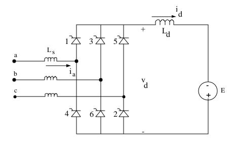
Nominal Values:  $V_{LL}(rms) = 480 \text{ V at } 60 \text{ Hz}$   $L_s = 1.0 \text{ mH}$   $L_d = 16 \text{ mH}, R_d = 1 \text{ ohm}$  E = 630 Vdelay angle  $\alpha = 160^\circ$
