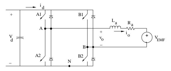
Nominal Values:  $V_d = 200 V$   $R_a = 0.37 \Omega$   $L_a = 1.5 mH$   $f_s = 10 \text{ kHz}$ , Unipolar Voltage Switching  $K_E = K_T = 0.75$
