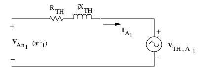
:.  $(V_{TH,A})_1 = 74.76 \ /-12.36^{\circ} V (rms)$
