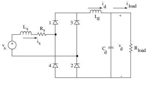
Nominal Values:  $V_{S}(rms) = 120V \text{ at } 60 \text{ Hz}$   $L_{s} = 1 \text{ mH}$   $R_{s} = 10 \text{ m}\Omega$   $L_{d} = 1\mu\text{H}$   $C_{d} = 1,000 \mu\text{F}$  $R_{load} = 20 \Omega$
