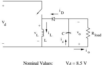
Values:  $V_d = 8.5 V$   $L = 10 \mu H$   $rL = 10 m\Omega$   $C = 100 \mu F$   $R_{load} = 8 \Omega$   $f_s = 100 \text{ kHz}$ switch duty ratio D = 0.75
