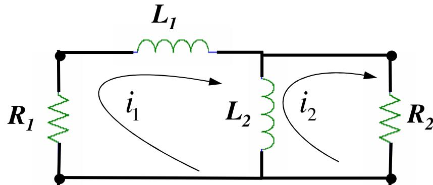
$$L_1 = 2H \quad L_2 = 3H \quad R_1 = 1\Omega \quad R_2 = 2\Omega$$
